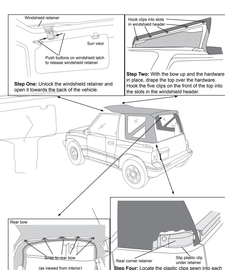
**Step Three:** Snap the five snaps on the inside of the top to the studs on the rear bow.
