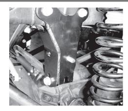
Step 3. Reinstall the track bar using the factory hardware in one of the two lower mounting holes which is suitable for the height of lift. Install the supplied 9/16 bolt with a washer on each side in the original track bar hole using the supplied spacer in the original trackbar mount location.
