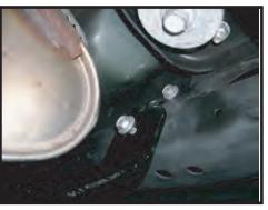
5. Install M12 Bolts and Washers through the Mounting Bracket and into the Skid Plate. Once all 3 have been started, tighten them.
