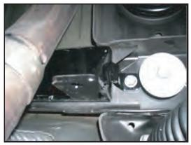
2010-2011 vehicles will need to use supplied M10 bolt, Washer and Nut Plate to install mounting bracket. Slide nut plate on top of frame cross member. Place M10 spacer between frame and mounting bracket. Insert M10 bolr and washer. Start bolt into nut plate but do not tighten.
