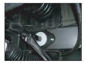
2. Slide the Mounting Brackets in between the frame and the exhaust. The muffler hangers may have to be removed to provide additional room. Position the mounting tabs of the Mounting Bracket onto the inner studs of the body mount. Replace nuts removed in Step 1, but do not tighten.
