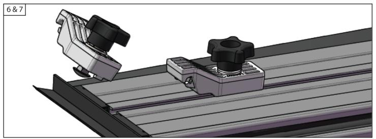
6 & 7. Slide the two front pre-staked cover retainer assemblies into the track on the underside of the tonneau cover, do not remove bolt from assembly.
