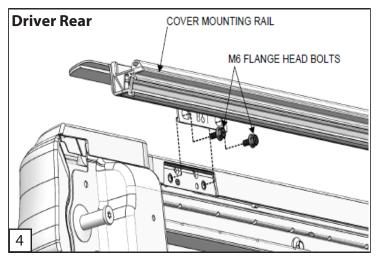
4. Install the rear portion of each mounting rail, using the M6 Flange head bolts and thread them into the pre-threaded holes located previously from the removed portion of the bed cap. Repeat process for opposite side. Leave bolts loose and proceed to step 5.
