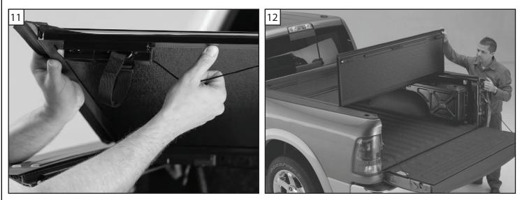
11 & 12. Once the cover is located correctly, fold the cover to the open position. Pull the release cables on the rear panel to release it from the side rail. Take care to fold it gently so the position of the cover is not disturbed.
