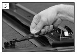
3, 4 & 5. If this is as far as you would like to open the cover, you can secure it in this position. Release the strap from the stowed position by squeezing the tabs. Attach the buckle at the bulkhead, pull the strap to take up the slack and secure the cover. Repeat this for the opposite side.
