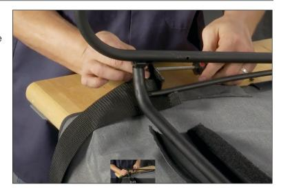
18. With both bows attached to the header and the center bow attached to the side bows, fold a portion of the Velcro and attach to the center bow. Do not attach the entire Velcro just a small portion in the middle to assist in installation. This will allow you the freedom to pull and adjust the top as needed. Once installed and adjusted you'll seal the entire Velcro strip.
