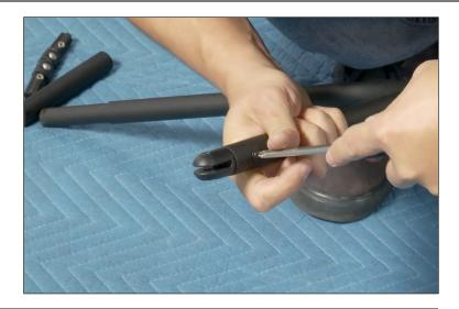
8. Insert the smaller "Dog Leg" Tube Frame piece into the main bow. Rotate to align the predrilled holes and fasten the two pieces with a screw.
