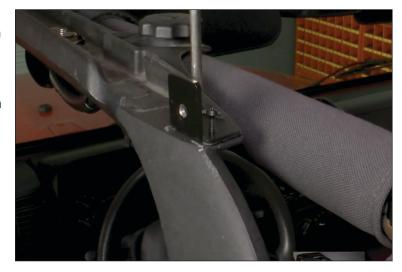
30. Bring the top forward and install the lanyard into the side bow to secure. Make sure lanyard is pushed all the through to avoid it rubbing with the top material.
