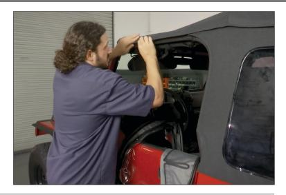
38. Slide rear window into rear tailgate bar. You'll notice a roll that slides into the channel of the tailgate bar.
