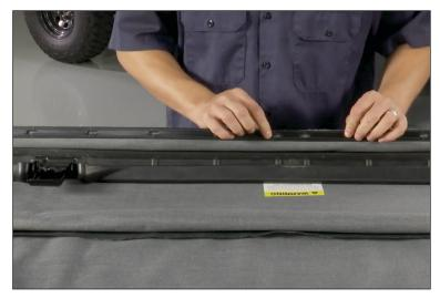
2. Now with the material holding into place take the header and flip it holding the material to the header. With this method it assure the attaching strip is in the appropriate position.
