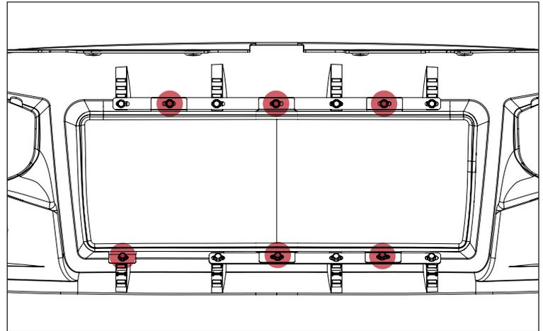
3. Install new grille insert using the M6 hardware from the previous step.
