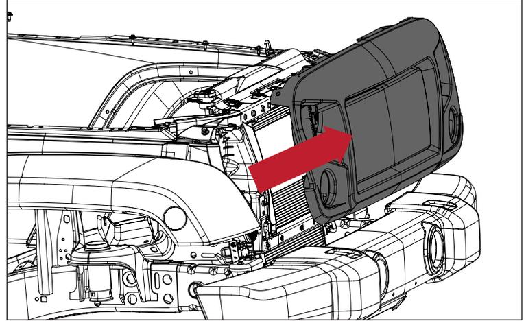
2. Remove highlighted M6 fasteners from rear of Spartan Grille. They will be reused for installing the LED insert. Remove mesh insert.
