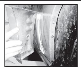
Step 4. Remove lower rocker panel cladding (if equipped).
