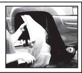
Step 6. Remove the inner wheel well sound dampening foam from the rear portion of the wheel well. Do not discard foam, it will be reused later. If any debris is present it must be removed before proceeding.
