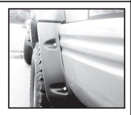
Step 52. Hold the assembled rear sections of flares against the body aligning the front area of the flare to the body crease behind the rear door opening. Adjust the flare to achieve a 1/4" gap between the wheel arch flare and the door flare.
