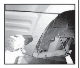
Step 59. Attach the L shaped brackets to the rear bumper cover as shown. The brackets will mount to the inside of the bumper cover and using a bolt and nut with a washer on each side of the bumper cover.
