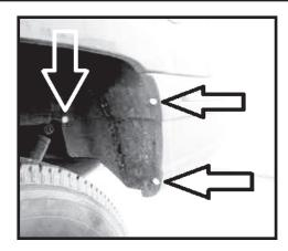
Step 56. Trim the rear bumper cover at the second line drawn using a sawzall or cut off wheel.
