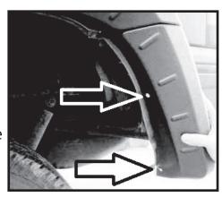
Step 58. Drill two mounting holes into the rear bumper cover using a 3/16" drill bit.
