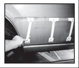
Step 44. Trim the retainer just below the upper clip portion and reinstall onto the door.
