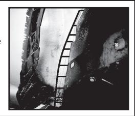
Step 14. Using a cutoff wheel or sawzall cut the lines made on the inner fender well. Cut only the horizontal lines from inside of the fender well to the vertical line drawn. Use caution when cutting. Do not over cut or cut into surrounding areas.
