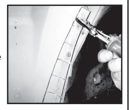
Step 11. Bend the tabs inward. The tabs should start at the line drawn and should be bent inward 90 degrees towards the fender well duplicating the factory bend.
