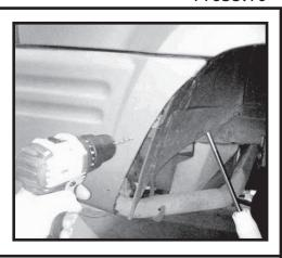
Step 62. Reinstall the rear bumper cover splash shield using the factory hardware previously removed. Attach the lower rear portion of the fender flare to the two L brackets on the rear bumper cover using two plastic push rivets.
