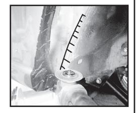
Step 15. Bend the cut tabs inward towards the fender well.
