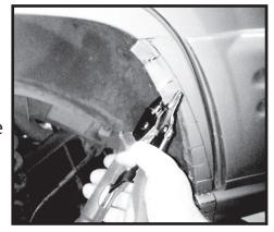
Step 36. Using a heavy hammer bend the tabs inward. The tabs should start at the line drawn and should be bent inward 90 degrees towards the fender well duplicating the factory bend.
