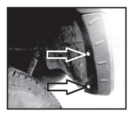
Step 63. Using a 3/32" drill bit, make pilot holes into the fender well using the pre-drilled holes in the fender flare as a guide.
