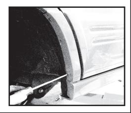
Step 32. If your vehicle is equipped with a plastic rocker panel cover, you will need to draw a vertical cut line and trim the cover. The line will need to start from the bottom point of the door trim and extend downward. A razor knife will be suitable for trimming. Ensure the cut is smooth, this area will be visible after the flare is installed. After trimming, the panel cover should be slid forward slightly or removed when cutting the body.
