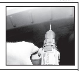
Step 26. Secure the flare to the wheel well using the supplied #8 screws. Do not over tighten screws.
