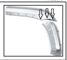
Step 50. Attach the rear and middle wheel arch flare sections using the supplied bolts and lock nuts with a washer on each side of the flare flange.
