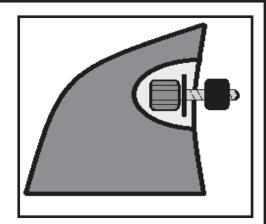
Step 23. Position flare against the body over the drilled mounting holes. Start each screw into the mounting holes. Once each screw has been started, snug the flare to the body. DO NOT TIGHTEN.
