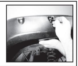
Step 46. Drill holes marked on fender using a 3/16" drill bit.
