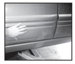
Step 48. Install the lower rear rocker panel end cover. Mark the mounting holes for the lower rear rocker panel end cover. The cover is held on with two self tapping screws on top and bottom of the cover and one body mounting bolt on the front.
