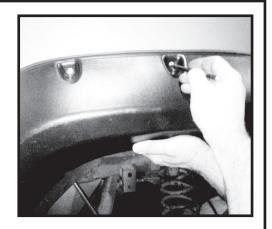
Step 20. Drill holes marked on fender using a 3/16" drill bit.
