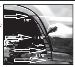
Step 34. Using a cutoff wheel or sawzall cut the lines made on the fender. Cut only the horizontal lines from inside of the fender to the vertical line drawn. Use caution when cutting. Do not over cut or cut into surrounding areas.
