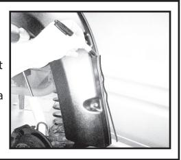
Step 40. Remove the retainer nut from the backside of the rear door that holds the lower body cladding on to the vehicle.
