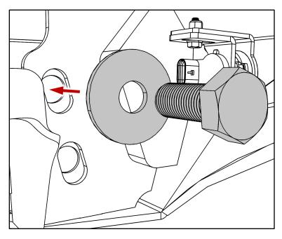
**12.** Install the shim plate on the driver side of the bumper at the two bottom mounting points (between the frame and the bumper). Repeat for the passenger side.
