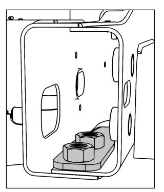
**10.** With a person lifting on each end, lift the bumper and align the bumper mounting holes with the mounting holes on the back of the Jeep frame.
