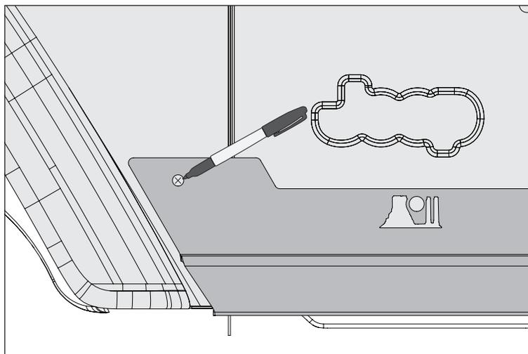
5. Beginning with a 3/16" bit, drill 6 mounting holes into side body. Continue with 7/16" bit for front 4 holes and 9/16" for rear 2 holes to finish full diameter of mounting points. Clean any metal chips and shavings from vehicle before continuing.
