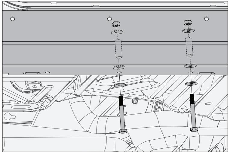
18. Attach Rock Slider Panels to 4 body mount tabs through 4 mounting slots using M6 Hex Bolts, M6 Large and Small Washers, and M6 Lock Nuts.
