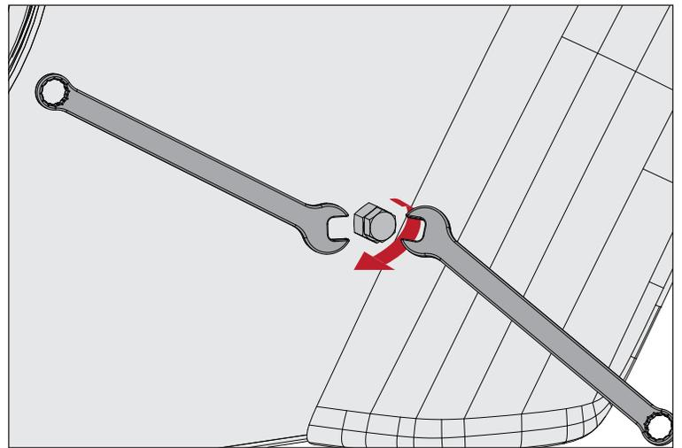
10. Install Rock Slider Panels to vehicle using M10 Button Head Bolts, M10 Flat Washers, and M10 Nuts.
