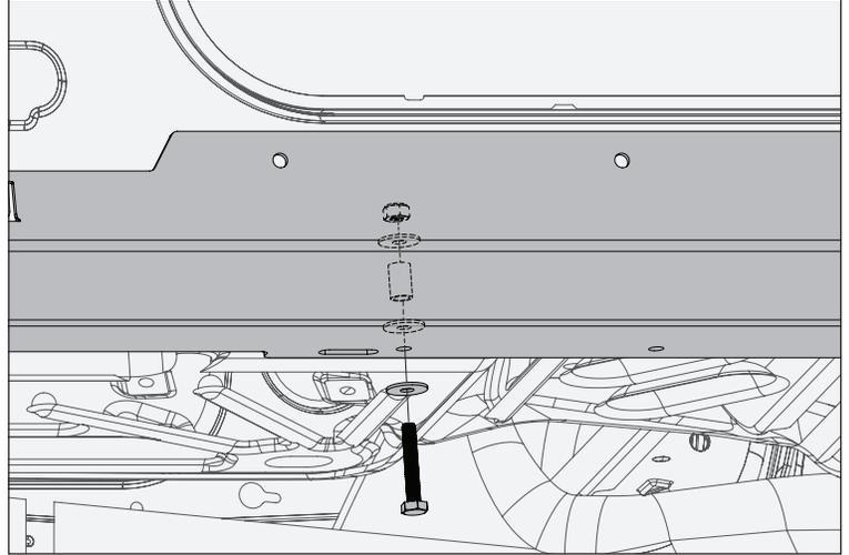
17. Attach remaining bottom holes using M10 Long Hex Head Bolt, Flat Washers, 45mm Spacer, and Lock Nuts.
