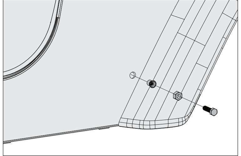
8. Using two wrenches to keep Hex Spacer Tool from spinning, tighten Hex Bolt Tool until Rivet Nut is fully collapsed.
