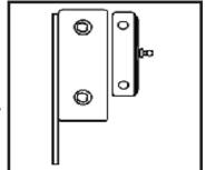
Step 2. With the supplied drill bit, you will need to drill the pilot holes using the marks made in the previous step. DO NOT drill through both sides of the hood. Only the bottom side off the hood should be penetrated. Use caution when drilling the pilot holes. Protective eye wear should be worn.
