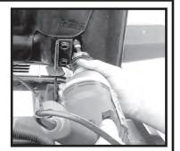
Step 3. Using two of the supplied screws and washers attach the bracket to the hood with the ball facing away from the engine compartment. Use caution when installing the screws. Over torquing can break the screws. Screws should be torqued to 25 in-lbs. Repeat for opposite side.
