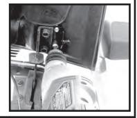
Step 4. Attach the hood lift shock to the bracket installed on the hood with the cartridge section facing upwards. Using the shock as a guide place a mounting bracket on the inner lip of the engine bay where the fender mounts. Position the bracket ball where it would be snapped into the shock. Mark the locations off the bracket holes. Repeat this step for the other side. Follow same procedures as in step 2 for attaching the bracket to the body.
