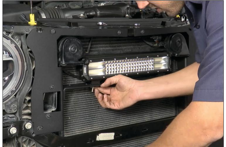
12. Lastly install the grille. Align the lower clips to the opening and push firmly on the face of the grille. Next install all the push-pin retainers along the top of the grille. This completes your install.
