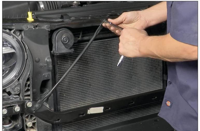
4. Now remove the plastic shield near each headlight. The passenger side will have more torx screws holding the air inlet, keep these screws. There are also push-in rivets that need to be pried out and removed. Remove each shield and disregard they will no longer be needed.
