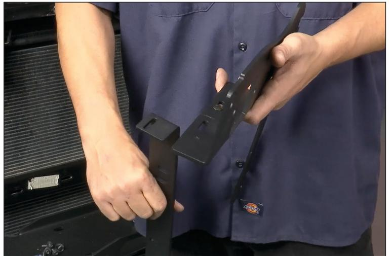
7. Place the passenger side bracket in place to the Jeep. Now use the hardware removed earlier to attach the bracket to the Jeep.
