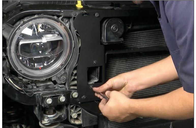
9. Attach the Drivers side light bracket to the Jeep. Just like the passenger side use the hardware removed to attach. The only difference is there is no air inlet tube to attach.
