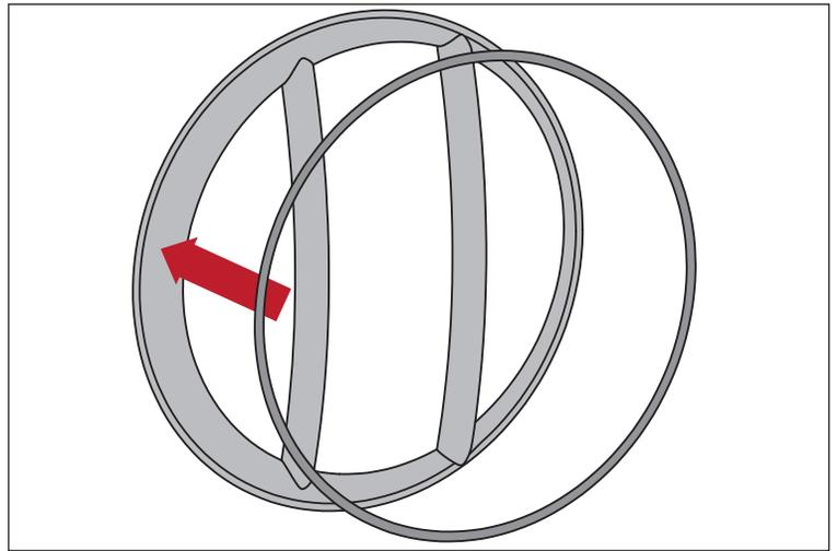
3. Insert Fog Light Guard into fog light opening. If applicable, O-Rings should contact bumper.
