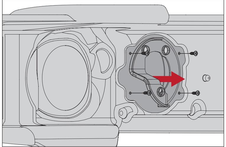
2. If using O-Ring, place around outside of Guard.
