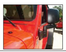
**Step 3.** Using the included hardare, install the relocation bracket using the existing factory door hinge bolt holes. Install both bolts loosely. Note that the relocation bracket points forward.
