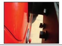
**Step 2.** Remove the two side door hinge bolts. The factory uses threadlock to retain these bolts, so some effort may be required.
