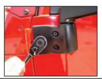
**Step 4.** Tighten both bolts snugly.
