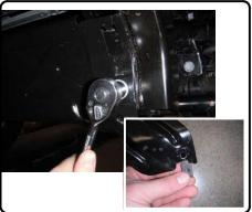
2) Raise hitch into position. Loosely install (4) 7/16" carriage bolts and spacers into the remaining mounting holes as shown above by inserting through the closest access hole. Use fishwire for the (2) rearmost bolts. If needed, add (1) or (2) 3/8" washers to each side between the rail and hitch to level the hitch. Install the supplied fascia tabs, (2) 10mm bolts and (2) conical washers thru the hole in hitch and 3/8" washer(s), if applicable, as shown above.
