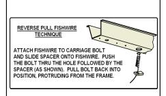
5. After fishwiring hardware into frame raise side plates and tow hooks into position and bolt to frame using spacers, 1/2"-13, and M12 hardware. (Finger tighten only).
