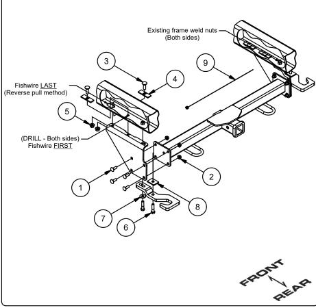
1. Remove tow hooks and set aside for later reattachment. Hardware to be returned to vehicle owner and will not be reused.
