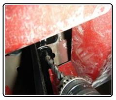
11. Remove side plates. Fishwire 1/2" carriage bolts and CM-SP40 spacers through drilled holes. Reverse fishwire 1/2" carrige bolts and CM-SP40 spacers into enlarged holes. (Reverse fishwiring hardware is not necessary if bumper removal was performed)
