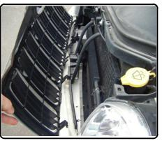
Begin the removal of front bumper cover by first removing the (2) lower screws from the bottom of bumper cover. Then remove (4) plastic fasteners from top of bumper cover.
