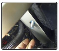
7. Locate and remove rubber plug located in lower grill on each side of the radiator.
