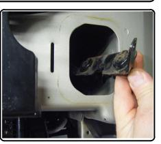
6. Fishwire (2) carriage bolts and spacers through the front of each frame rail and out middle round hole and rear square hole, as shown
