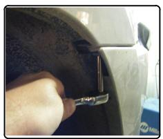
4. Remove factory tow hooks and lock nuts. These will not be reinstalled and should be returned to vehicle owner.
