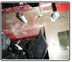
12. Install side plates and secure with 1/2" hex flange nuts.
