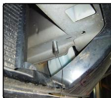
12. Reverse fishwire 1/2" carriage bolt and CM-SP17 spacer into rear mounting hole on each side.
