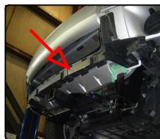
16. If removed in step 1, raise air dam into position and mark location to trim for receiver tube. After hole is trimmed for the receiver tube, raise air dam back into position and mark trim locations for the hitch chain loops (See below). Trim dimensions are approximate. Check fit prior to trimming. Reinstall air dam.
