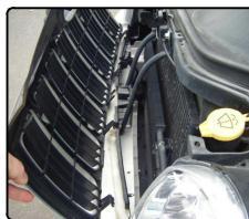
4. Begin the removal of front bumper cover by first removing the (3) lower screws from the bottom of bumper cover.
