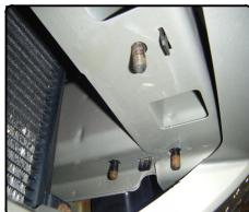
8. Remove the front frame end caps to allow removal of factory installed tow hook hardware.
