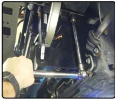
14. On 2010 models, trim fascia so it is able to be fastened back onto vehicle cross member. (See TRIM DIAGRAM below) Trim dimensions are approximate. Check fit prior trimming.
