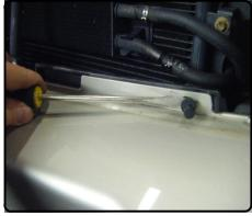
5. Continue bumper cover removal by removing (2) plastic fasteners and (1) socket screw in each wheel well.
