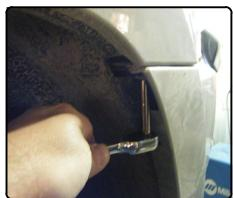
6. Carefully pull bumper away from frame. Twist and remove head light lamps from their housing units. Place bumper off to the side.
