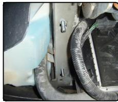
13. Using the fishwires on the carriage bolts as a guide raise hitch into position. (Rubber guards will need to be temporarily flipped out of the way on 2010 models) Remove the fishwires and secure with flange nuts.
