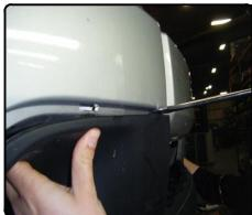
2. Remove air dam by removing (5) plastic fasteners. If optional trimming is selected this will occur in step 18.
