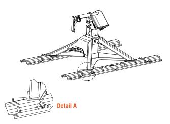
If installing new base rails, follow the instructions provided by the rail manufacturer for proper placement, alignment and spacing per your vehicle's year, make and model. If the 5th wheel is being mounted to existing base rails, and alignment issues arise, it may be necessary to proceed as follows:
