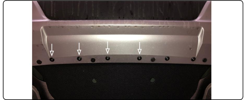
6. Remove (2) fasteners located inside bumper cover to allow rear fascia to flex. Trim fascia and wire track using aviation shears as shown in trim diagram. Avoid cutting sensor wires by moving it out of the wire track.
