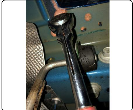
**RUBBER ISOLATOR REMOVAL DIAGRAM**
