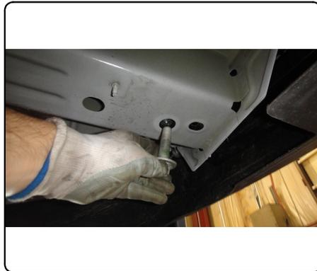
5. If kick sensor is present, remove (4) of the (6) rivets using a drill along rear fascia, starting from driver side, to avoid damaging kick sensor while trimming. Replacement rivets are included.
