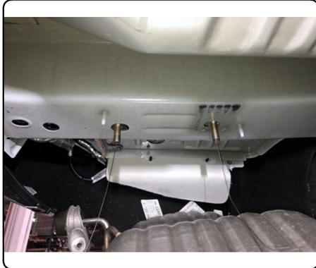
8. Raise hitch into position. (**NOTE:** Hitch will be positioned between the upper and lower kick sensor wires if equipped as shown in step 9.) Torque 1/2" hardware to 75 ft-lbs and torque M16 hardware to 146 ft-lbs.
