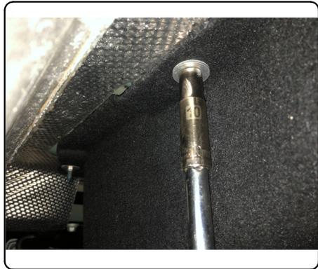
2. Lower exhaust by removing (1) fastener on outside of frame rail, on each side, using 10mm socket. Remove (2) exhaust isolator hangers by using Rubber Isolator Removal Diagram as reference.
