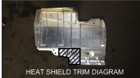
4. Remove (2) push pins from the rear fascia, bend push pin mounting tabs away from the rear of the vehicle to allow space to raise hitch into place. Mark and trim the rear fascia, using the trim diagram as a reference.
