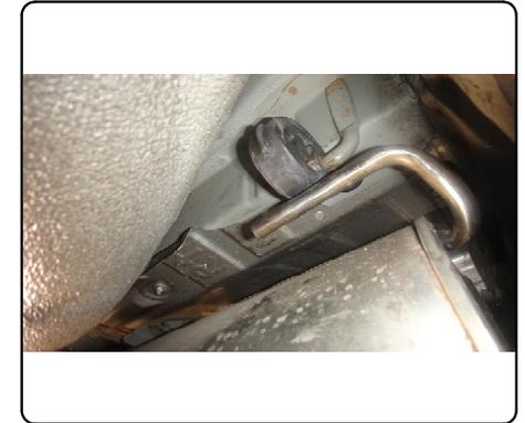
2. Remove (4) heat shield screws with phillips head screwdriver or 10mm socket (both sides if equipped with dual exhaust). Remove four hole plugs from each side of frame to expose mounting holes. Return all hole plugs to customer.
