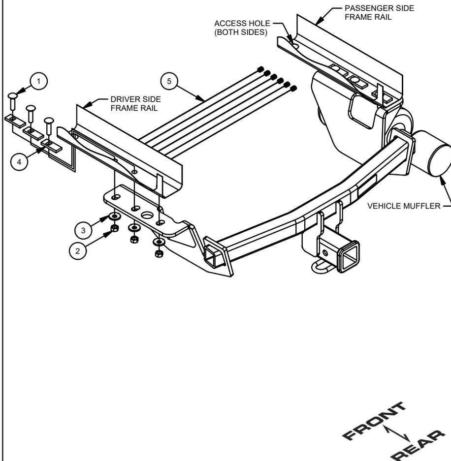
1. Remove (2) exhaust hangers from the passenger side muffler and (1) exhaust hanger from the center-front of vehicle for single exhaust vehicles, dual exhaust will remove (2) hangers from the driver side muffler as well. Support lowered exhaust with jack stand.
