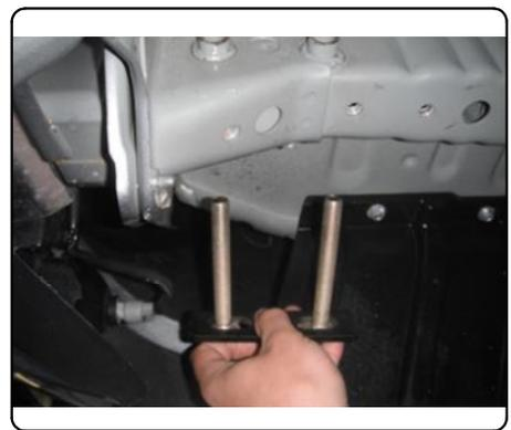
3. Raise hitch into position and slide the bolts through to support it. Loosely install the (4) supplied 1/2" hex flange nuts and the (2) hex bolts and conical washers as shown. Be sure teeth on washers are against the hitch mounting plate.
