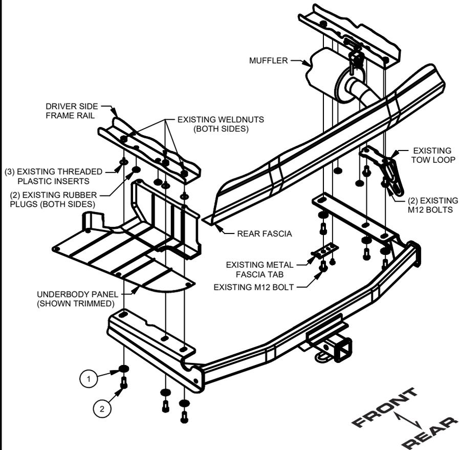
1. Remove the (7) fasteners securing the driver side underbody panel. After lowering the underbody panel return it to the owner or trim and reinstall in Step (7).
