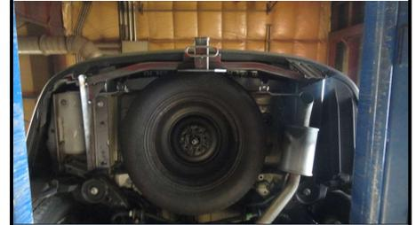
7. Mark and trim underbody panel. Reattach underbody panel using fasteners removed in Step (1). Note: See underbody panel trim diagram. Dimensions are approximate, confirm fit prior to trimming. Use ribs of the underbody panel as cutting guides.
