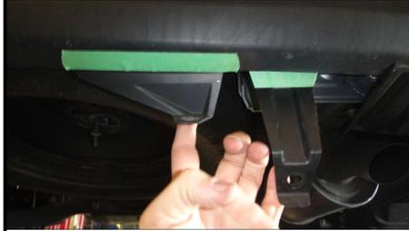
5. Remove the (3) M12 bolts securing the metal fascia tab and tow loop to the passenger side frame rail. Remove the (1) fascia screw and metal fascia tab from the passenger side underbody panel. Return the fascia tab, tow loop, and fasteners to owner.
