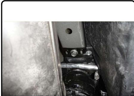
6. Raise the hitch over the exhaust and align the holes in the hitch with the weldnuts in the frame. Secure the hitch to the frame using the supplied M12-1.25 hex bolts and 1/2" conical toothed washers. Torque all 12mm hardware to 86 ft-lbs.
