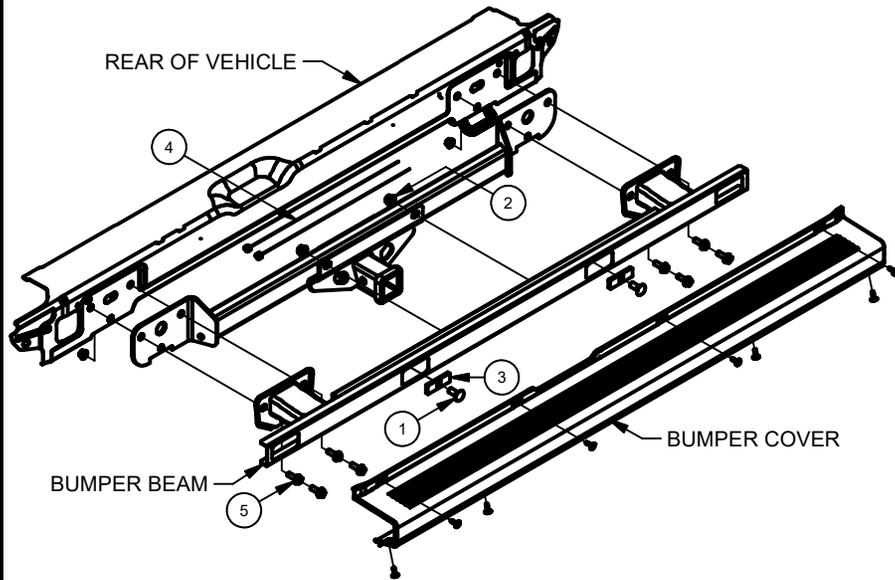
1. Open the rear vehicle doors to expose the bumper cover and fasteners. Using a T30 torxbit, remove (8) fasteners and the bumper cover. **Note:** If present, disconnect the rear back-up sensor before completely removing the bumper cover.
