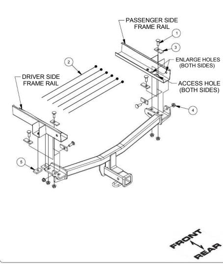
1. Remove (2) fasteners centered along the bottom of the rear bumper cover using a T27 socket.
