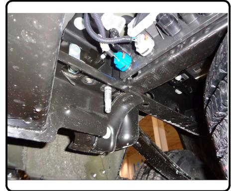
2. Install 1/2" carriage bolts, spacers, and flange nuts in remaining holes as shown. Torque all 1/2" hardware to 110 ft-lbs. Torque all M14 hardware to 103 ft-lbs. Raise spare tire if lowered during install.
