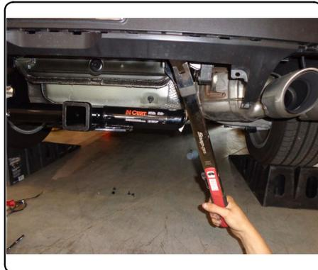
9. **Porsche models:** Raise rear fascia up into position and mark around side plate interference where fascia needs to be trimmed. Approx. 1/2" by 1" each side. Trim area with either a cut-off wheel or shears. After fit is confirmed, clip fascia back into position by following Steps 1-2 in reverse.
