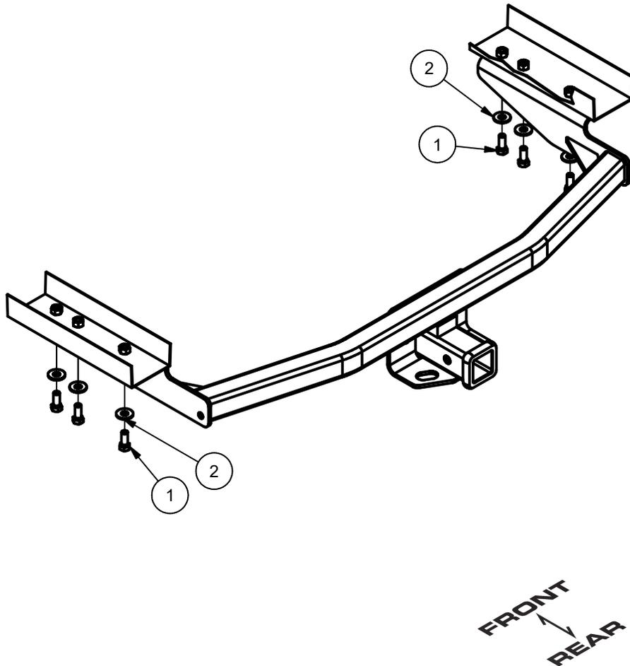
1. Remove tow hook from driver side frame rail. Return tow hook and fasteners to vehicle owner.
