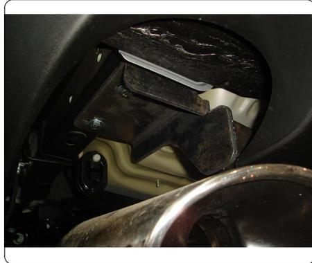
4. Torque all M10 fasteners to 48 ft-lbs.
