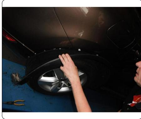
4. Remove (4) torx head fasteners from under wheel well trim.
