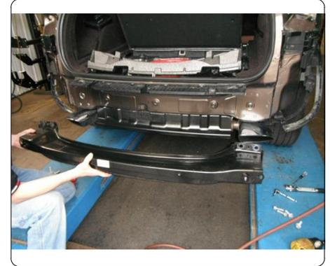
9. Install the hitch using the M12 bolts removed in step 8. Foam insert can be discarded or trimmed and reinstalled. **Note:** Trim foam so it loosely fits into position.
