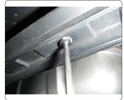
2. Remove mud flap from behind each rear tire by unfastening (5) torx head screws from each. **Note:** Underside fasteners have a nut attached.
