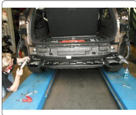
8. Remove foam insert. Remove bumper beam by unfastening (8) M12 bolts. These bolts will be used to install the hitch. Return bumper beam to vehicle owner.
