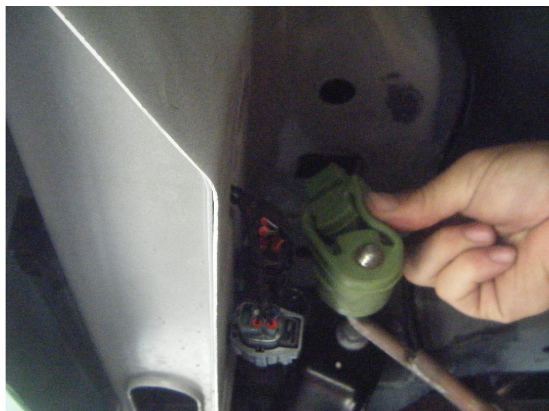
EXHAUST HANGER REMOVAL
