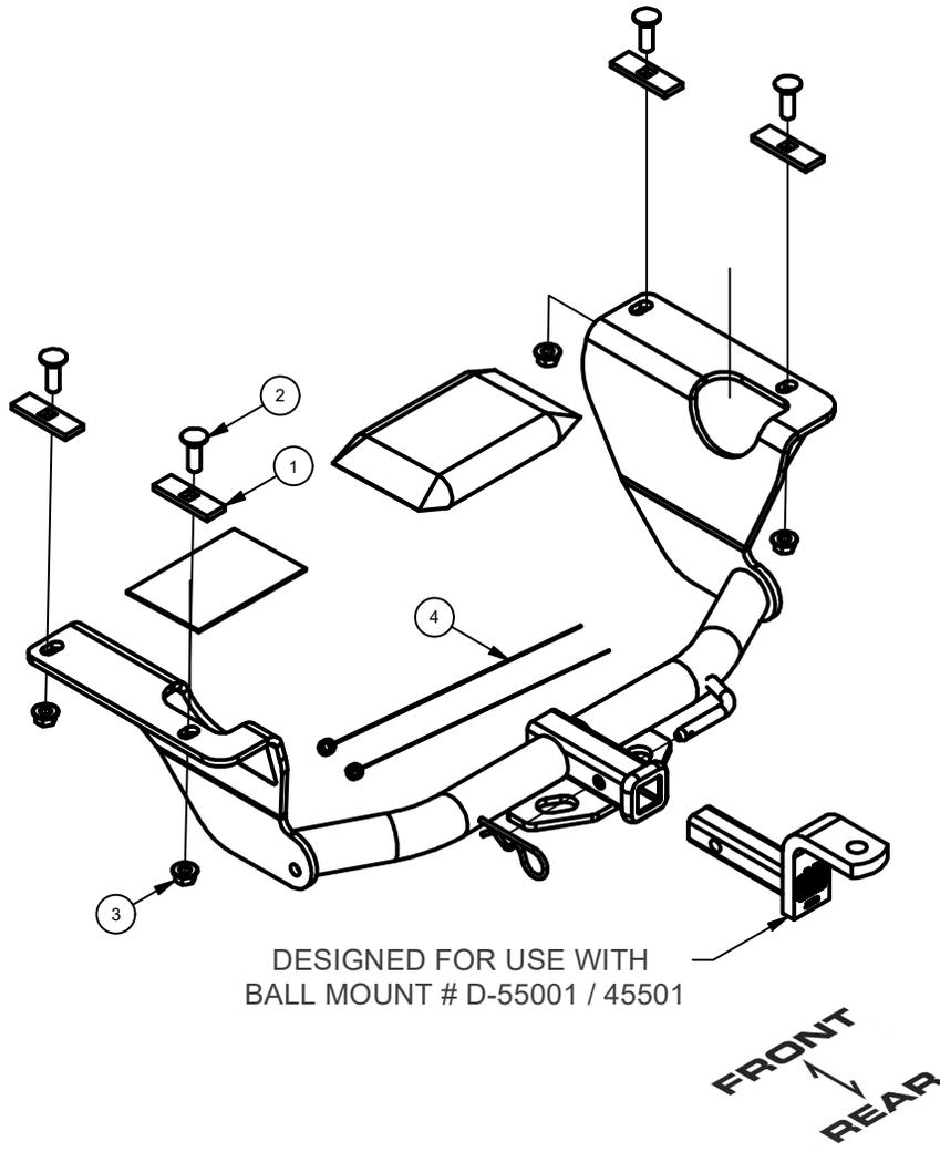
1. Remove (2) rearmost rubber isolators from exhaust muffler. One isolator is located towards outside of vehicle and one is located towards inside of vehicle.
