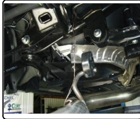
5. Trim heat shield with aviation shears according to diagram.
