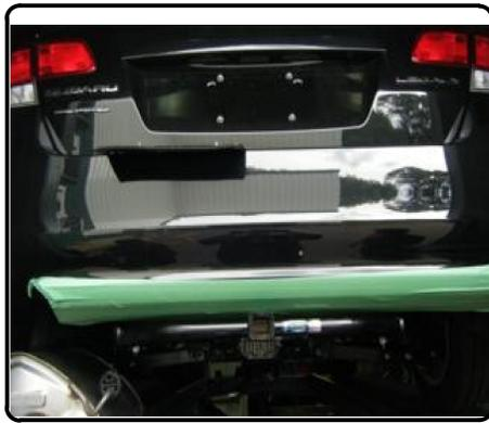
13. Reinstall trimmed heat shield with (3) screws saved from Step 4. Use 10mm socket to tighten heat shield screws.
