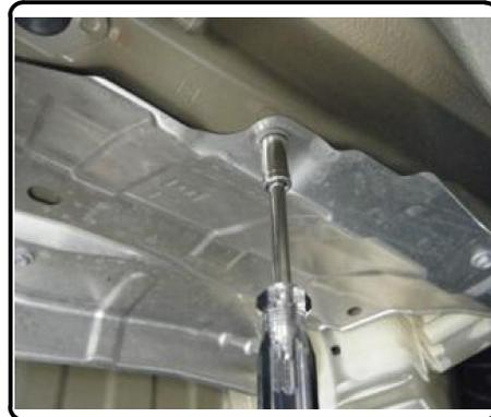
6. Remove (4) rubber plugs from frame rails. (2) plugs per frame rail. Discard plugs.
