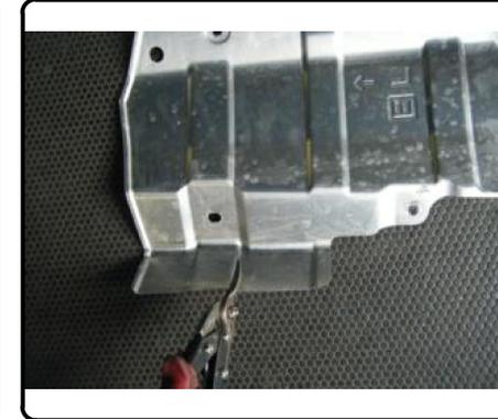
4. Remove (4) screws from vehicle heat shield with 10mm socket. Remove heat shield from vehicle. Save screws for reinstallation in Step 13. Save heat shield for trimming and reinstallation.
