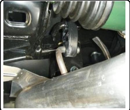
**RUBBER ISOLATOR REMOVAL DIAGRAM**
