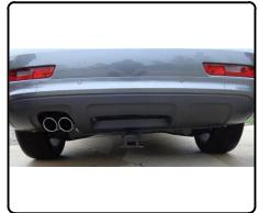
8. Trim a 2-1/2" square section from the center at the bottom of the bumper fascia using aviation shears.
