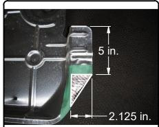
4. Enlarge the attachment holes along the bottom of each frame rail and the hole on the outside of each frame rail. Fishwire 1/2" carriage bolts and SP10 spacers through the access hole to the forwardmost hole and outside holes on each frame rail.
