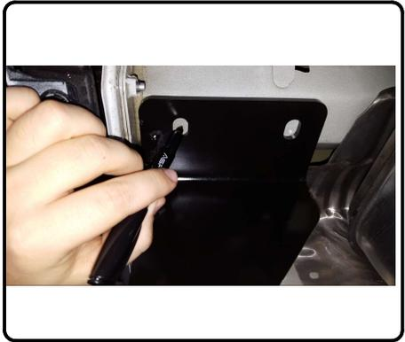
2. Lower the hitch and use a drill and 1/4" drill bit to drill (4) holes located at the marked areas from step 1. Then, use a 1/2" drill bit to open up the holes to the final size.
