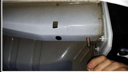
5. Using the forward-most holes that were enlarged in step 3, reverse fishwire (2) 7/16" carriage bolts and (2) CM-SP7 spacers into the frame. (See reverse fishwire diagram).
