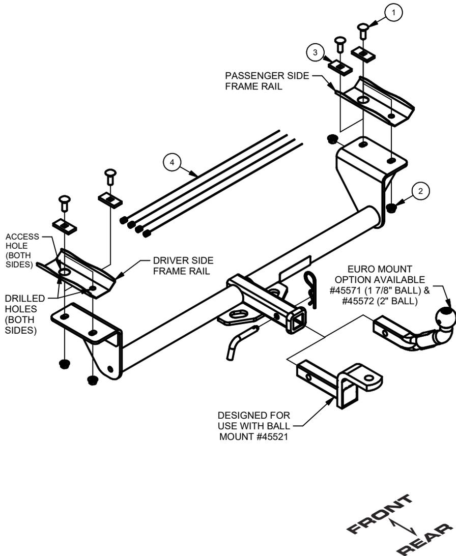
1. Raise hitch into position against the back of the frame rail. Using the hitch as a template, center the holes on the frame rail and use a paint pen to mark out the (4) hole locations.
