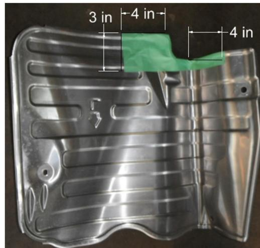
HEAT SHIELD TRIMMING DIAGRAM
