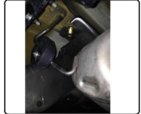
6. Torque 3/8" fasteners to 43 lb-ft and all 7/16" fasteners to 59 lb-ft.
