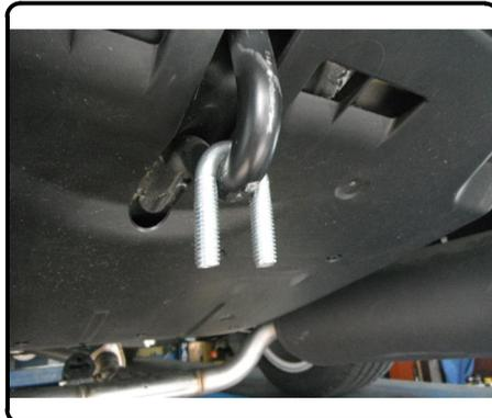
5. Raise hitch into position. Secure to U-bolt with 3/8" hex flange nuts. Remove fishwires and attach 7/16" hex nuts to carriage bolts.
