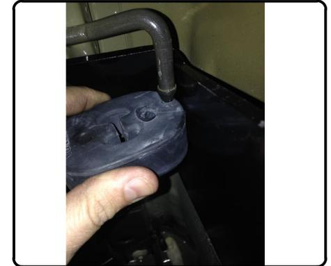
2. Remove heat shield by removing (2) bolts per shield.
