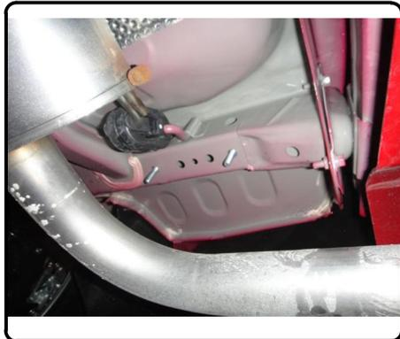
3. Raise the hitch into position with the tow loop above the hitch and secure to vehicle with carriage bolts, spacers and flange nuts as shown.
