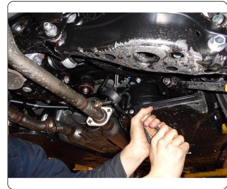
2. Remove the (6) hex flange bolts securing the exhaust hanger brackets with a 17mm socket and remove the brackets (each side). Save the bolts and brackets for reassembly.
