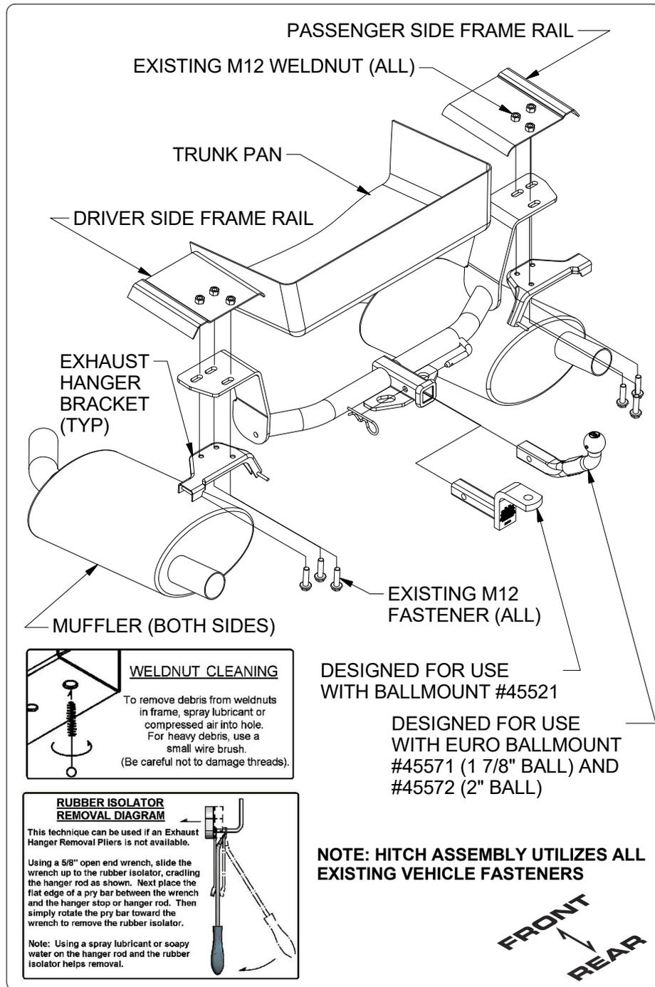
1. Lower the exhaust by removing (2) rubber isolators from the hanger bracket on each muffler. Also remove (2) forward center isolators allowing the exhaust to hang below frame rail (support exhaust from underneath).
