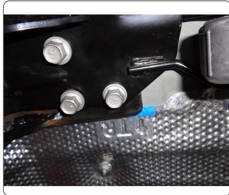
4. Raise the hitch into position against the frame rails and reinstall the exhaust hanger brackets using the (6) M12 bolts. Note: The hitch is sandwiched between the frame rails and the exhaust hanger bolts.
