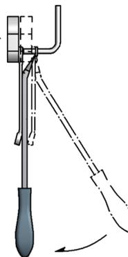
This technique can be used if an Exhaust Hanger Removal Pliers is not available.
