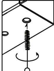
To remove debris from weldnuts in frame, spray lubricant or compressed air into hole. For heavy debris, use a small wire brush. (Be careful not to damage threads).
