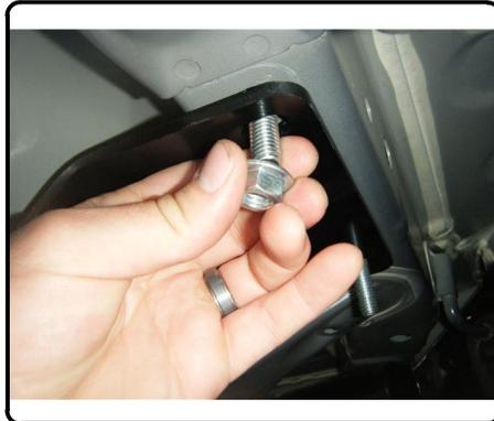
5. Fishwire remaining hardware through enlarged access hole and out the side of frame rail and tabs on hitch. Secure with flange nuts. Torque all 1/2" fasteners to 110 lb-ft. (Both sides)
