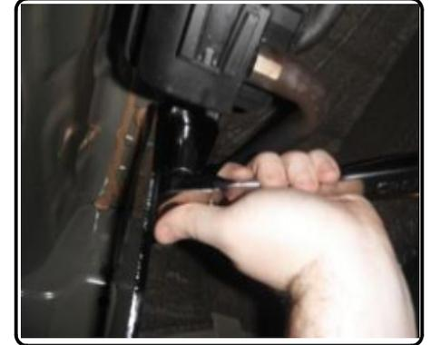
6. Raise exhaust back into position and reattach the rubber isolators. Install is complete.
