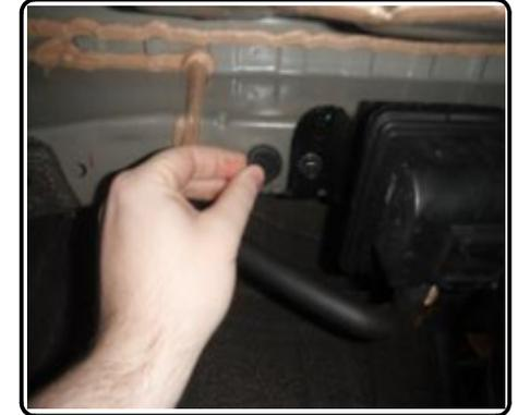
2. Trim heat shield to allow access to round hole on passenger side of vehicle.
