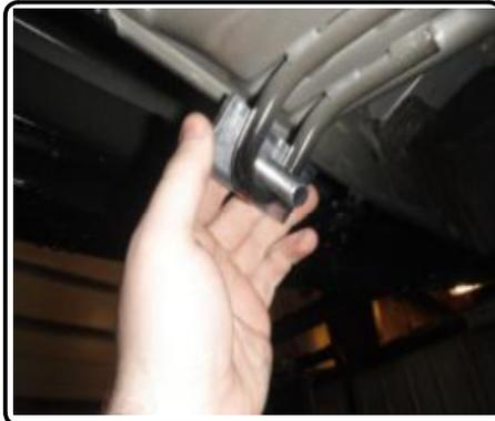
5. Raise hitch into position and secure with 1/2" hex flange nuts. Torque 1/2" hardware to 110 lb-ft.
