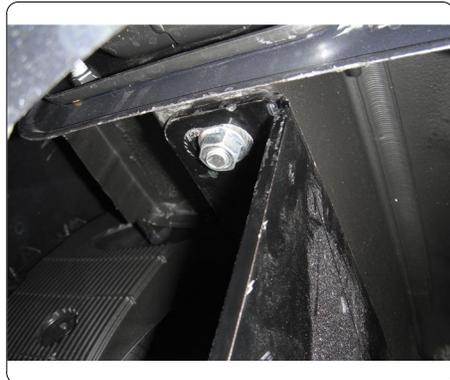
5. Install the remaining 3/8" hardware with (1) CM-SP34 spacer onto the vehicle tow loop, as shown above.
