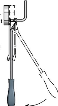
This technique can be used if and Exhaust Hanger Removal Pliers is not available.
