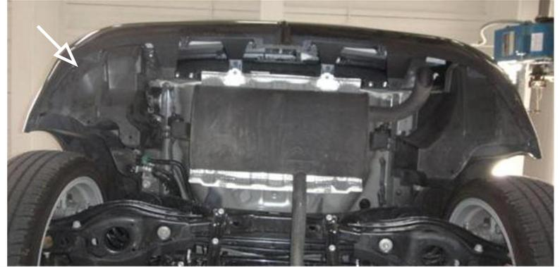
2. Remove (2) tow loop bolts and tow loop. Return tow loop and bolts to owner. **Note:** The first photo shows the tow loop covered by the underbody panel, the second shows the underbody panel removed.
