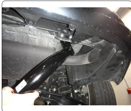
4. Torque all M12 hardware to 86 ft-lbs. Reinstall underbody panel removed in Step (1).
