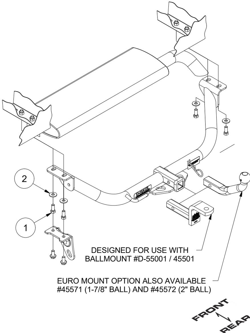
1. Remove the driver side underbody panel by removing (5) fasteners. Panel and fasteners will be reinstated later.
