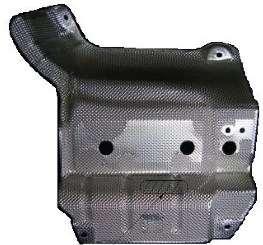
AREA TO TRIM MUFFLER HEAT SHIELD TRIMMING DIAGRAM
