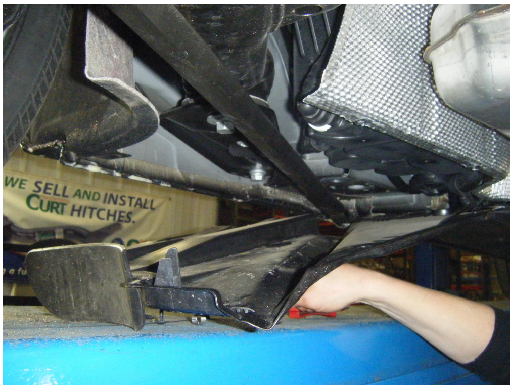
PLASTIC COVER REMOVAL (CONVERTIBLES ONLY)
