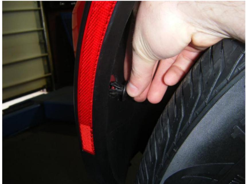
3. Pull the fender flair away from the bumper cover to access the (2) hidden fasteners, one each side. Using an offset phillips screwdriver remove the hex head screw.
