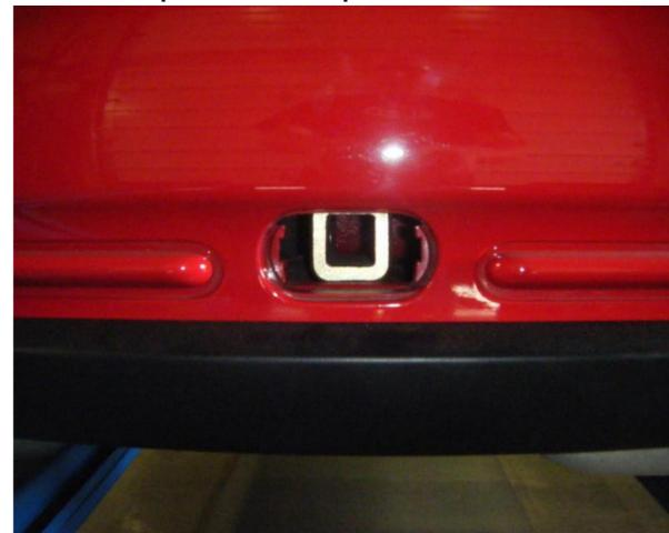
12. Align bumper cover and pull back on the fender flairs. Re-attach wiring harness to bumper cover. **Note:** Side markers need to be re-attached to the wire harness prior to securing bumper cover. Reinstall all (11) fasteners removed previously and snap fender flairs back into place.
