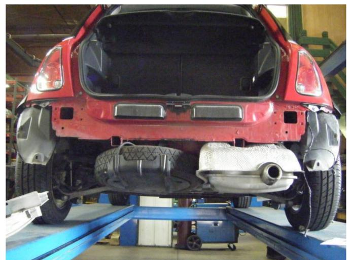
9. Raise the hitch into position by aligning the holes with the weldnuts. **Note:** The hitch will fit firmly between the spare tire and the rear panel.
