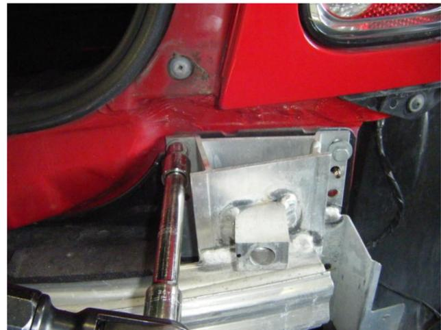
8. Remove the (2) plastic nuts securing the divider panel to the aluminum bumper beam. Return the plastic nuts, divider panel, and hard foam energy absorber to owner.
