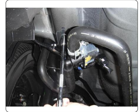
2. Lower exhaust by removing (2) rubber isolators from the hangers attached to the frame.
