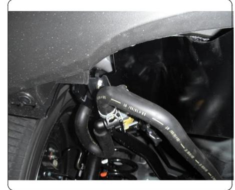
6. Torque all 7/16" hardware to 70 ft-lbs. Torque all 1/4" hardware to 12 ft-lbs. Raise exhaust back into position. Installation is now complete.
