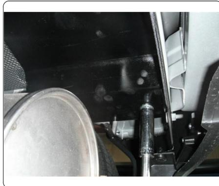
5. Place the 1/4-20 x 1" carriage bolt through the square hole in the driver side plate. Attach the vapor canister lowered in Step (1) to the carriage bolt and secure with the 1/4-20 flange nut.
