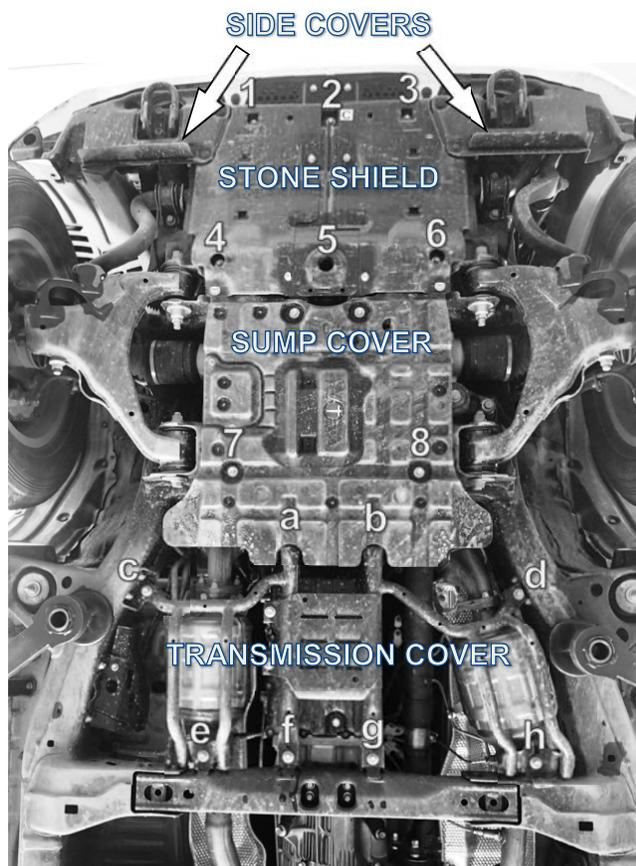
Factory under vehicle protection on car
