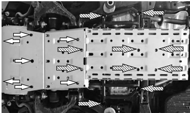
**Tighten M8 & M10 hardware to vehicle**
