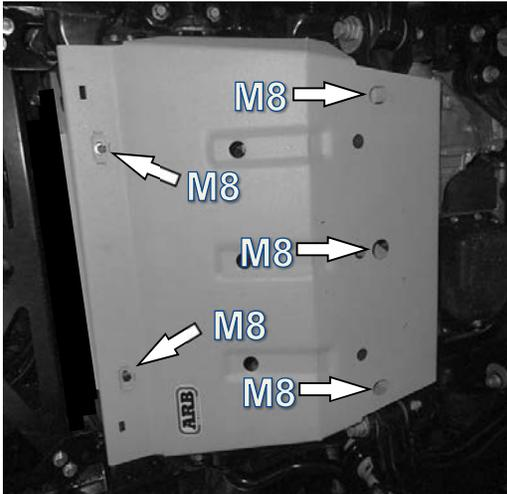
Fit front panel to vehicle
