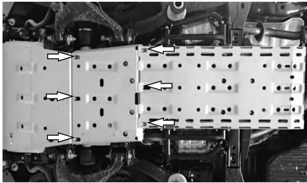
**Tighten M8 fasteners connecting each Panel**
