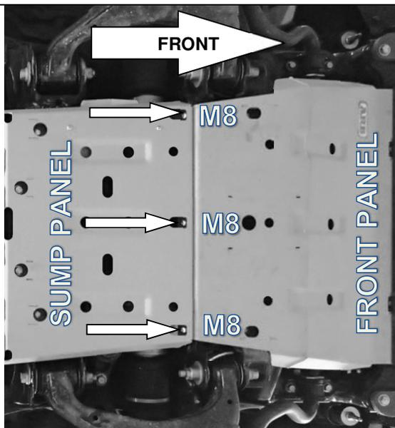
**Fasten Sump Panel to Front Panel**
