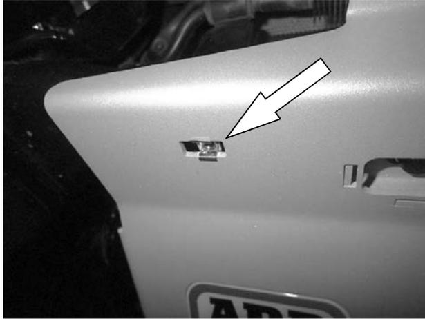
Fit cage nuts to front panel
