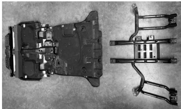
Factory under vehicle protection - REMOVED
