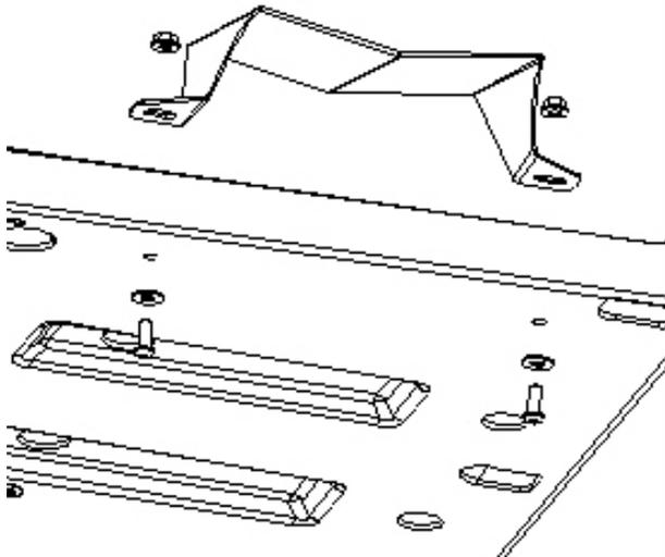
Fasten oil drainage bracket to diff panel
