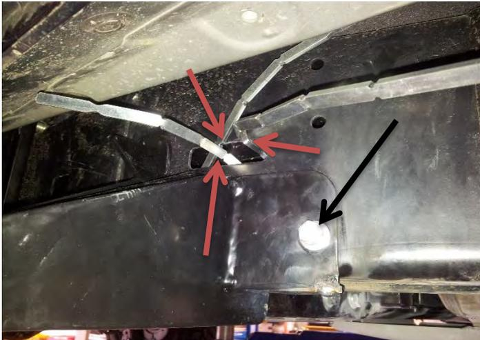
30. Bend 2 x M8 nut plates so they can be inserted into chassis rail. Align these with the 10mm holes in the side of the rail and start M8 x 40 bolts with spring and flat washers. Trim tabs with side cutters at red arrows and insure tabs do not rattle on chassis. (RHS shown)
