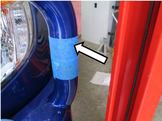
2. Use masking tape to wrap **1 x layer only** of tape around the Bull Bar Outer Frame to protect it from damage. Ensure masking tape is applied flat and without creases.
