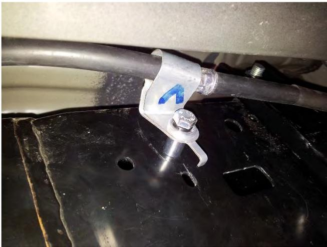
27. Re-fit the LHS front hand brake cable with the M8 x 50 bolt with spring and flat washers. Add the 19 mm long spacer to the bolt as shown to clear the side rail mount.
