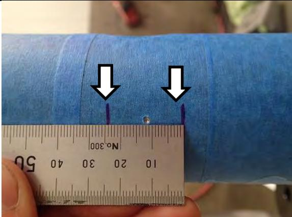
23. Using a marker pen, mark the outer frame 12mm above and below the Centre Punch mark (12mm + 12mm = 24mm).
