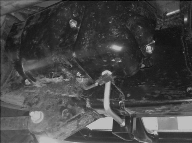
26. Re-fit the rear KDSS unit - cover in reverse order to removal as shown.(If fitted)
