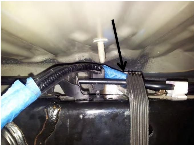
28. On the RHS, locate the front U-bolt behind the transmission cross member, ensure the U-bolt is placed under the lines on top of the chassis rail as shown.
