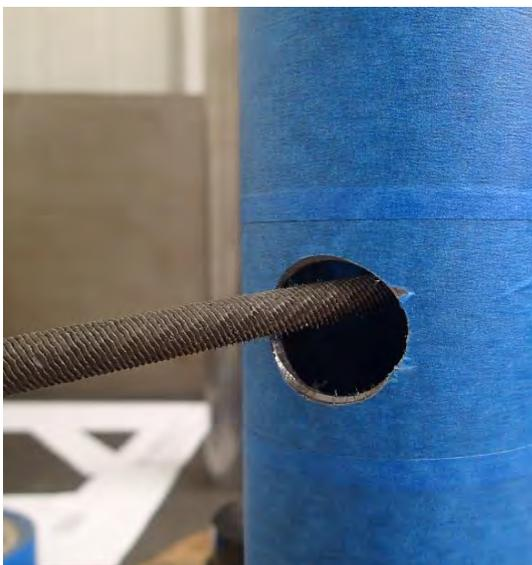
27. Using a small Round or Half-Round File carefully remove any burrs from the edge of the  $\text{\O}24\text{mm}$  hole.
