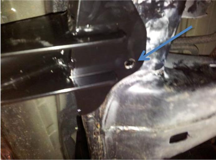
20. Bend M12 cage nut plate so it can be inserted into chassis rail .Align with the square hole in the bottom of chassis rail and start M12 x 40 bolt with spring and flat washers.(RHS shown)
