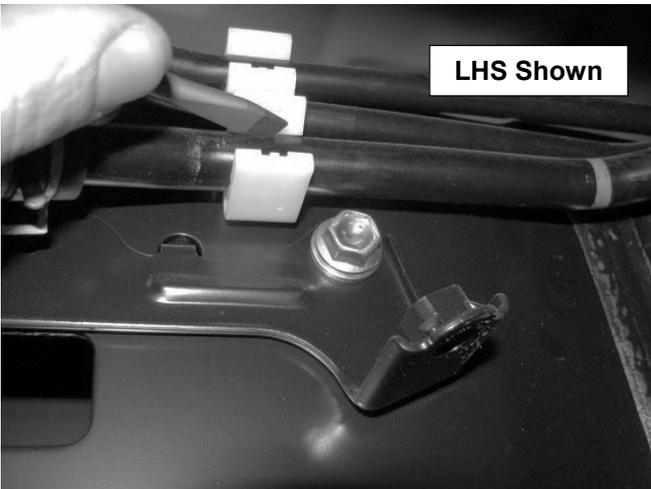
6. Unclip the lines from the chassis connector under the brake line cover. Use a screw driver to depress the plastic lock tabs carefully pulling the lines free as shown.
