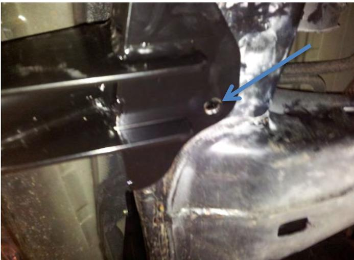
31. Bend M12 cage nut plate so it can be inserted into chassis rail. Align with the square hole in the bottom of chassis rail and start M12 x 40 bolt with spring and flat washers.(RHS shown)
