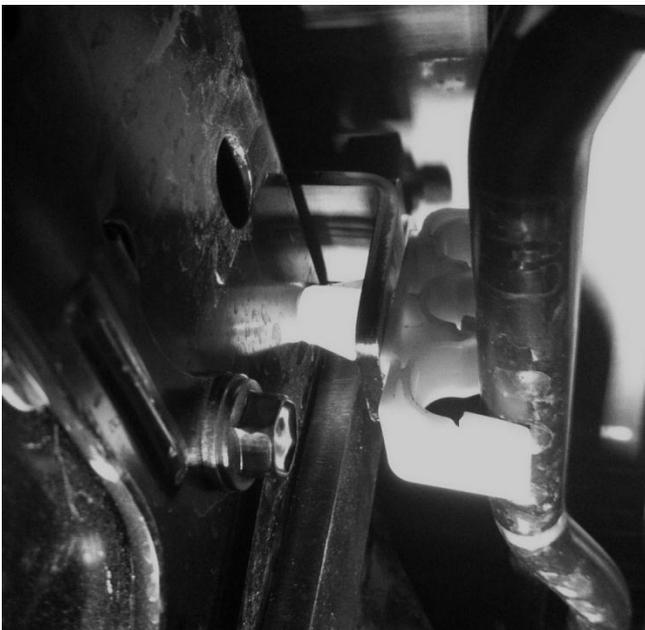
25. Fit the chassis line connector to the top bracket in reverse order to removal as shown. Clip the lines into position.
