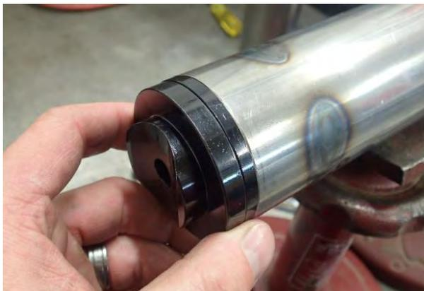
18. Swing the Side Rail outwards and away from the vehicle allowing installation of appropriate/selected spacer into gap between the front end of the Side Rail and the Tube Spigot. (5mm in this instance).
