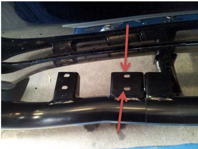
43. Slots indicated by red arrows are not used in this assembly to fix tread plates down. There are no holes in the tread plates to align with these slots. Use front mount bracket only.
