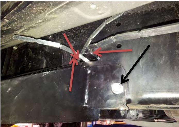
19. Bend 2 x M8 nut plates so they can be inserted into chassis rail. Align these with the 10mm holes in the side of the rail and start M8 x 40 bolts with spring and flat washers. Trim tabs with side cutters at red arrows to insure tabs do not rattle on chassis. (RHS shown)
