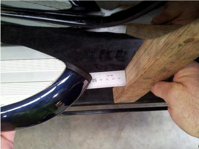
24. Adjust side rail to the nominal fore and aft position by aligning the rear wheel arch with a straight edge and measuring 50mm forward of the rear tangent line of the side rail.
