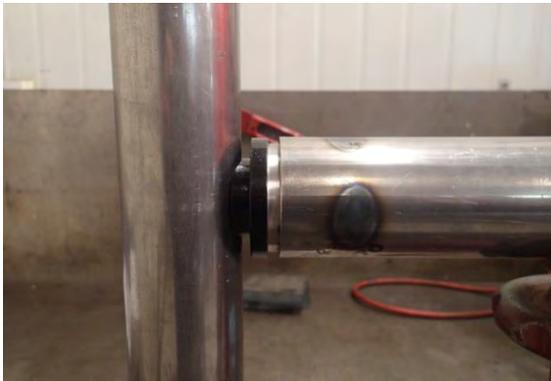
5. Hold Side Rail so that when viewed from the side of the vehicle the top tube is horizontal (**parallel to the ground**) and the Side Rail sits as desired against the side of the vehicle.
