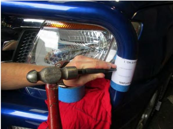
20. Using a Centre Punch, carefully Centre Punch the outer frame at the centre mark of “TEMPLATE 1”.
