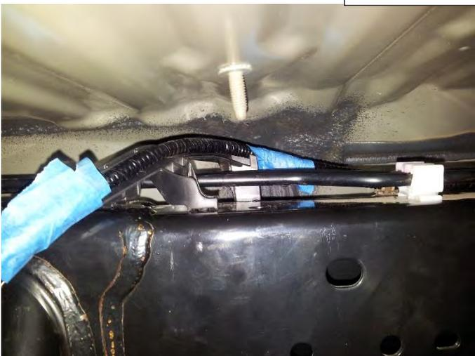
10. **KDSS\*** - Remove and discard the two bolts and the chassis/body block from the top of the LHS chassis rail located 200 mm in front of the rear tyre as shown.
