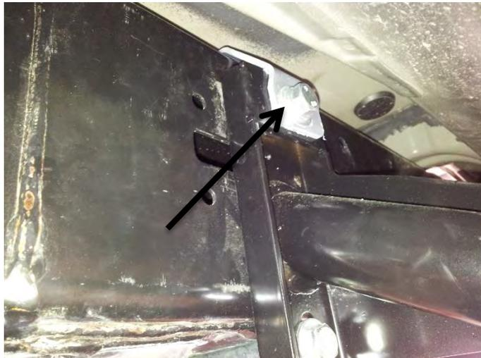
21. Place the top chassis bracket over the rail mount and start M12 x 25mm bolt with spring and flat washer.
