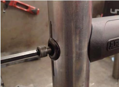
37. Install Submerged Bush and M10 Bolt.
