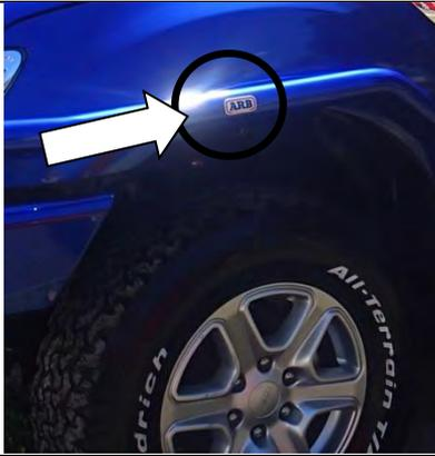
46. If fitting front rails, apply the supplied ARB decals here on both the RH and LH sides of the vehicle.
