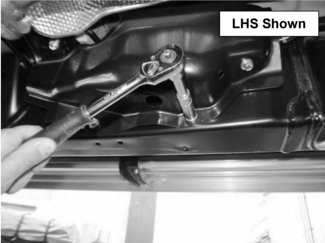
5. On the left hand side (LHS), inner side of the chassis & behind the transmission cross member, remove the brake line cover as shown.
