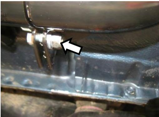
38. Tighten M8 Bolt ensure the slot and holes in the 6250024- SPACER S/STEP / RETURN LG RAD are aligned with the holes in the Step / Side Rail Brackets.
