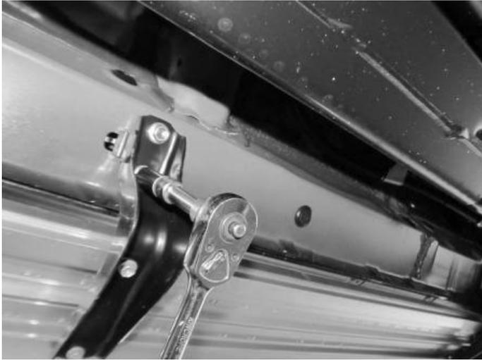
1. Remove and discard factory side steps by removing six M8 bolts per side as shown.
