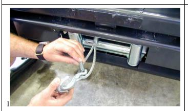
15. Feed the winch cable through the roller fair lead .
