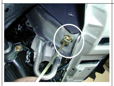
4. The three bolts that hold the washer bottle need to be removed to provide clear access to the chassis.
