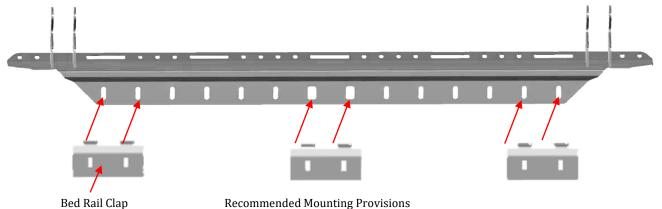
The feet on the XRS rack have a series of holes to allow for mounting in different locations. It is recommended to install the plates on the outer sides of the feet as well as in the center. This will help distribute clamping force
