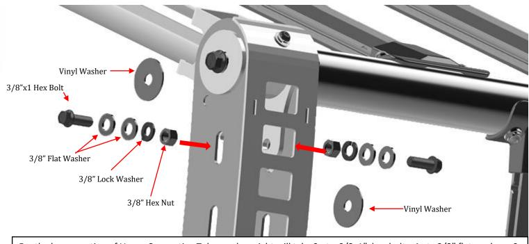
For the lower section of Upper Connecting Tube, each upright will take 2 qty. 3/8x1" hex bolts, 4 qty 3/8" flat washers, 2 lock washers, 2 hex nuts. Leave finger tight and repeat process for the remaining three corners. Install the hex bolt from the outside of the upright with one flat washer. On the inside of the upright, you'll need to install the 1 ½" vinyl spacers in between, then install one 3/8 flat washer, one 3/8 lock washer and one 3/8 hex nut. Repeat process for each upper corner.
