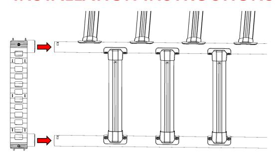
Connect vertical uprights to upper and lower connecting tubes. Identify that you have the top (single weep hole) and bottom (two weep hole) in the correct position.
