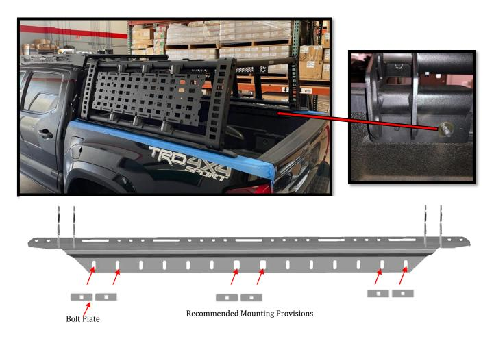
The feet on the XRS rack have a series of holes to allow for mounting in different locations. It is recommended to install the plates on the outer sides of the feet as well as in the center. This will help distribute clamping force.
