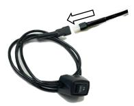
**Step 24:** Locate the black wires for the disable switch and feed them to your desired mount location. Prepare the surface by cleaning with a 50/50 mix of isopropyl alcohol and water or equivalent. Once the surface is dry, peel the backing from the double-sided tape and stick the disable switch on the lower dash panel. Plug the disable switch connector into the black wire harness and tuck the extra wire behind the lower dash panel.
