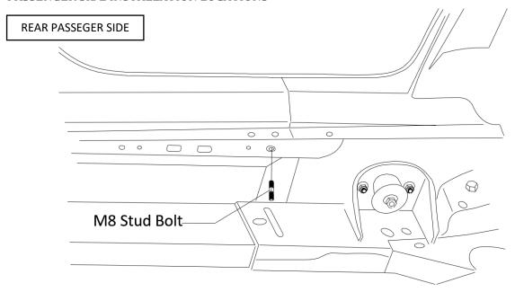
Step 3: : Install the rear passenger side motor mounting bracket using an M8 stud bolt
