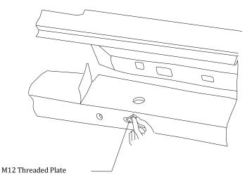
**Step 10**: Locate elongated hole opening on the front of the frame (bottom of the frame) and insert the M12 threaded plate and align thread with hole on the bottom side of the frame.
