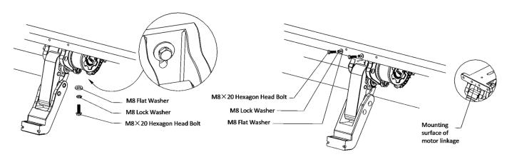
**Step 7**: . Install rear passenger side bracket onto weld seam using (2) M8x20MM Hex Bolts, M8 Lock Washer, M8 Flat Washer. On the underside of the bracket, secure it to the motor to the mounting plate using (1) M8x20MM Hex Bolts, M8 Lock Washer, M8 Flat Washer.
