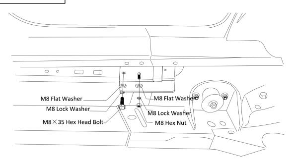
**Step 4**: Install the rear passenger side motor mounting plate using M8x35 Hex Bolt (1), M8 Lock Washer (1), M8 Flat Washer (1) on the exposed threaded hole. On the M8 Threaded Stud, fasten it with m8 Hex Nut (1), M8 Lock Washer (1), M8 Flat Washer (1). Torque down to 17 FT LBS.
