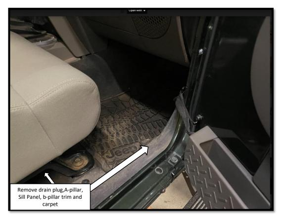
**Step 19:** Go under the vehicle and feed the door trigger signal wires (white and brown) and the disable switch wires (two black wires) into the cab. Feed the wires thru the hole in the rubber drain plug. Pop the drain plug back into the slot. Seal around the wires using RTV silicone adhesive to prevent water intrusion.
