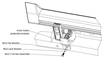
**Step 11**: Install the passenger side front motor protective bracket. Secure the protective bracket using an M12 hex bolt, flat washer, and lock washer. Torque to 25 ft-lbs.
