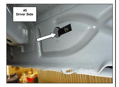
**Step-4** Attach one of the driver side brackets to the rocker panel using the U-Nut, (1) M8 hex bolt, (1) 5/16" lock washer and (1) 5/16" flat washer, and to the pinch mold using (1) M8 hex bolt, (2) 5/16" flat washers, (1) 5/16" lock washer, and (1) M8 hex nut. Leave the nut and bolts loose for final adjustment, **(Photo 6)**.
